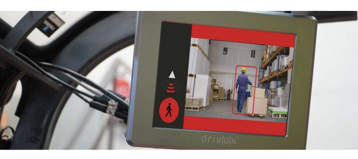
**Drivox**® is a product based on **AI** technology (Artificial Intelligence through neural networks) from Xesol Innovation. It is a safety system for industrial vehicles that detects and differentiates pedestrians from objects, alerting the operator by means of a visual and audible alert in case of potential risk of collision.
